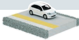
Thin Polyurethane Flooring System Fully Exposed
